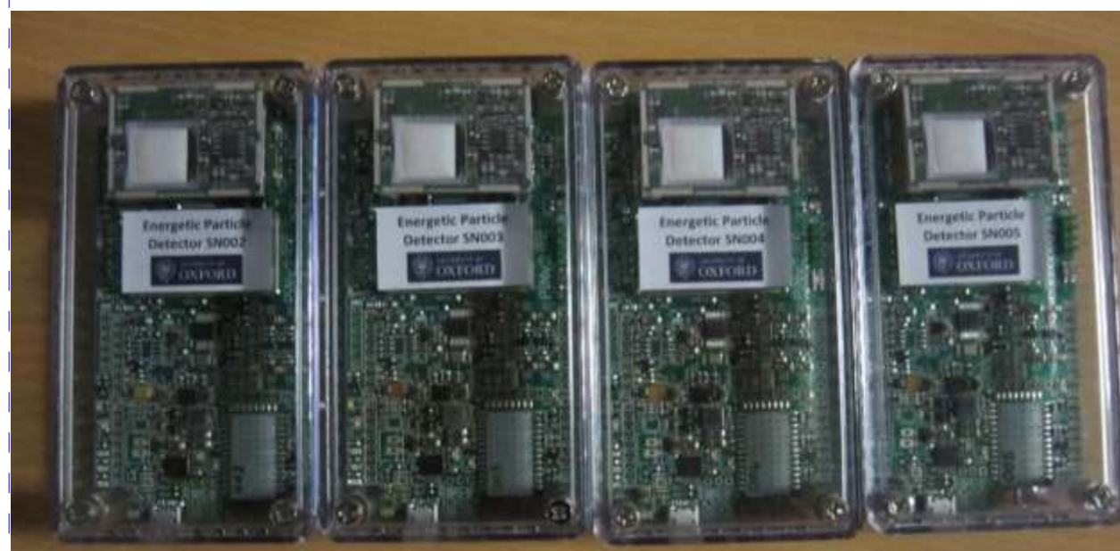
Example of current developments in miniaturised atmospheric electricity sensors. New hand held radioactivity/cosmic ray detector developed by the University of Oxford, UK, giving particle counts and energy and suitable for use on a variety of platforms including ground based networks, balloons and aircraft. http://www2.physics.ox.ac.uk/news/2017/12/20/wireless-radiation-detector-new-invention .
