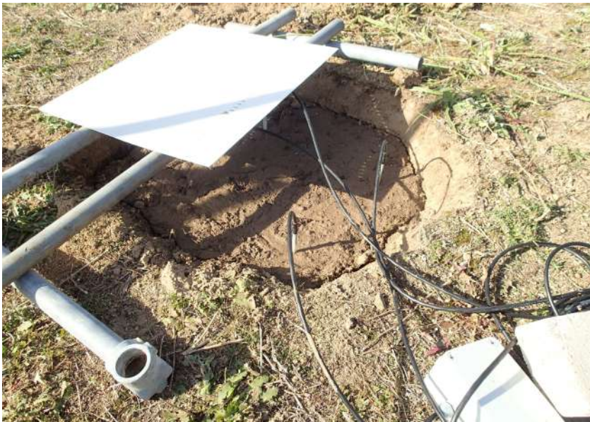
Figure 3.4: Applied shielding of two probes. Metal plate was connected to ground (green/yellow GND wire).
