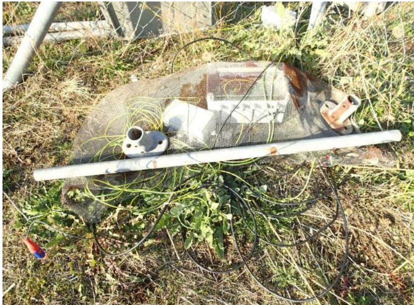
Figure 3.5: Setup in second week. Hypnos and junction boxes under grounded mesh wire. Reference located in bottom left (red top).
