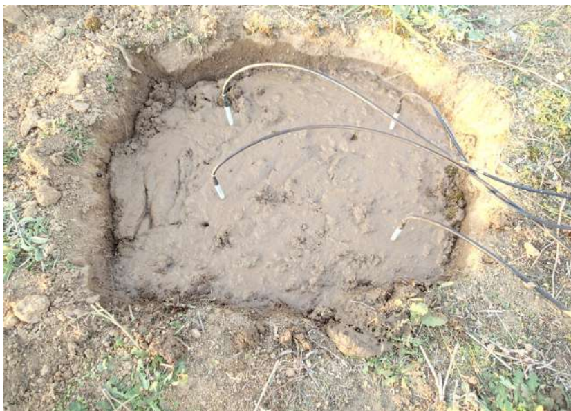
Figure 3.3: Probes placed in the mud inside the hole.
