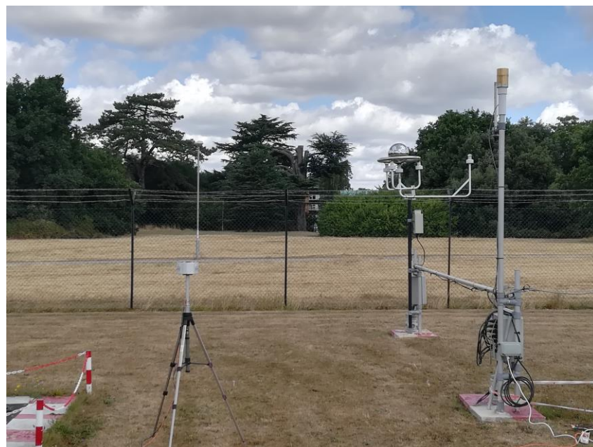
Fig. 2. Photo of the portable BOLTEK EFM 100 and the JCI131 field mills.
