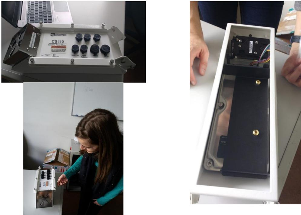
Fig. 1. Campbell Scientific CS110 Electric Field Meter Sensor
